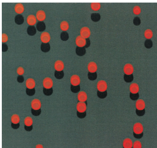
Figure 2 A three-dimensional CLSM image showing both surface and optical section at midplane of the FITC-labeled aminated poly(GMA) particles. [Color figure can be viewed in the online issue, which is available at www.interscience.wiley.com .]
